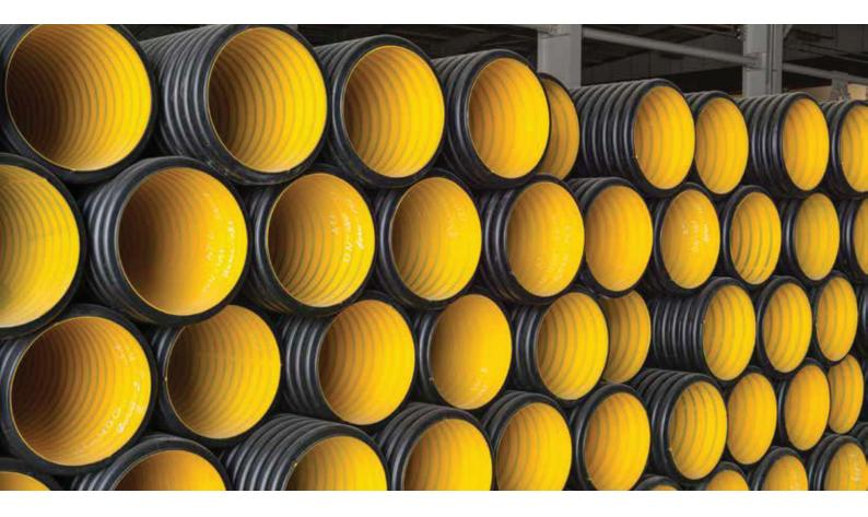
Double corrugated polyethylene pipes (corrugated pipes) are primarily produced in diameters 100DN-600DN. The inner side of the double corrugated pipes are made of flat layer from high-density polyethylene (HDPE) and exterior layer is corrugated. Inner wall can be tailor-made in yellow, white and blue colors according to the customer's wishes.
